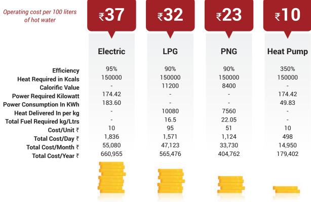
Above Calculations are based on following Data Quantity of Hot water Estimated (Liters.) 5000; Cold Water Inlet Temperature (20°C); Hot water Temperature (50°C)
