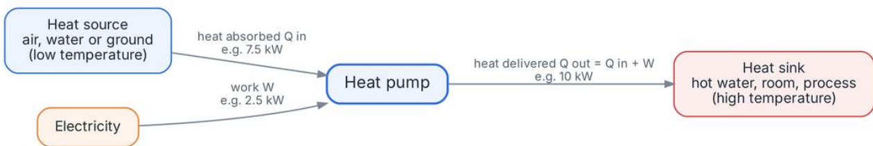
Energy flow through a heat pump
